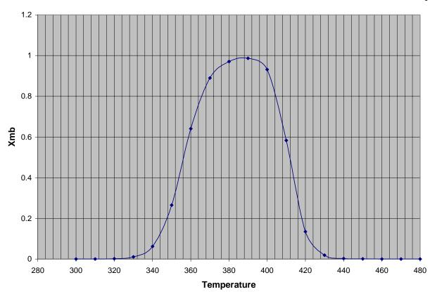
$$X_{\it EB} = \frac{U\!A(T-T_a)/F_{A0} + \tilde{C}_{\it pA}(T-T_0)}{-\Delta H_{\it Rx}} \ \ {\rm is \ the \ energy \ balance \ equation.} \ \ {\rm Superimpose \ on \ the \ curve \ given.}$$
