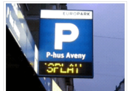
An information sign outside a parking garage in Sweden. The blinking effect is due to the rapid multiplexing of each LED row.
