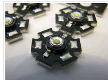
High-power light emitting diodes (Luxeon, Lumileds)
