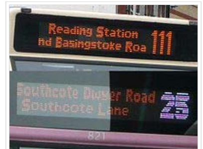
LED destination displays on buses, one with a colored route number.
