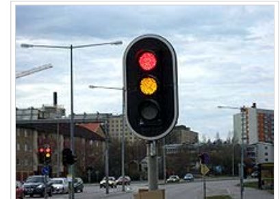
Red, yellow and green (unlit) LEDs used in a traffic signal in Sweden.
