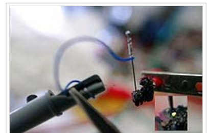
Green electroluminescence from a point contact on a crystal of SiC recreates H. J. Round's original experiment from 1907.
