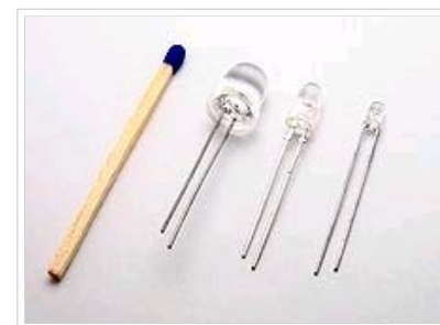
Different sized LEDs. 8 mm, 5 mm and 3 mm, with a wooden match-stick for scale.
