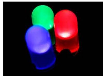
Red, green and blue LEDs of the 5mm type
