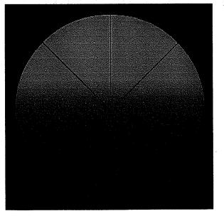
If you are close to the index of refraction of your sample you should see that the view in the eyepiece shows a dark region on the bottom and a lighter region on the top.
