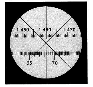
To read the index of refraction, depress the switch on the left hand side of the refractometer until you see the scale through the eyepiece. The upper scale indicates the index of refraction. By carefully interpolating you can read the value to 4 decimal place accuracy. The example shown here has a refractive index of 1.4606.
