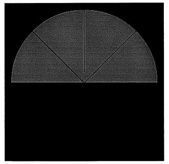
Once you have a crisp demarcation between the light and dark regions, turn the handwheel on the right hand side to place the borderline exactly on the center of the crosshairs as shown.
