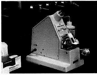
Some labs store the refractometer with a piece of tissue in the prism assembly to keep the prism glass from being scratched.
