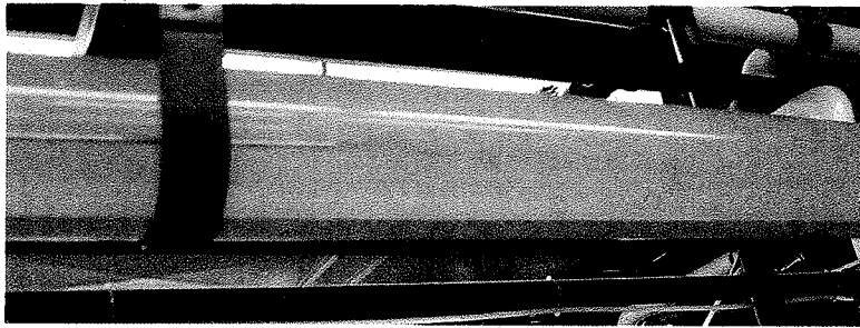
Figure E-10. Photograph of site-glass pipe used for visible inspection of flow type.
